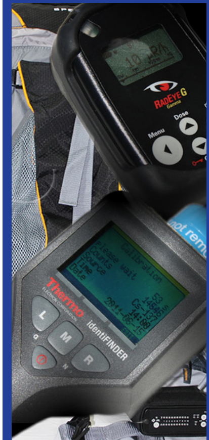
Instruments used for detection and identification of radiological materials taught in this course—CTOS/NNSA
