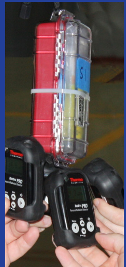
Students take radiation readings using a PRD-CTOS/ NNSA
