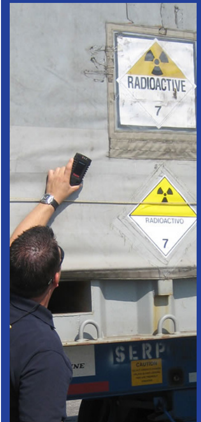
Performing a primary level screening on a trailer hauling radioactive materials
